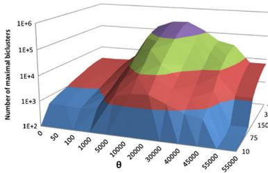
(i) Numbers of patterns (Y-axis) w.r.t.  $\theta$  (X-axis) and  $|G|$  (Z-axis)
